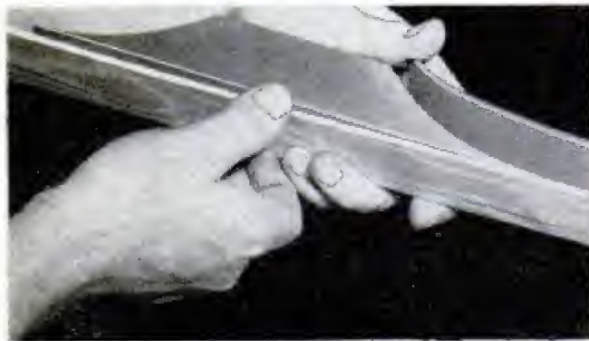
Above, the lemonwood lamination follows curve of the riser and is tapered to 1/64-in. thickness at the end. Below, professional bowmakers use a special bending jig of this type for bending recurve tips
